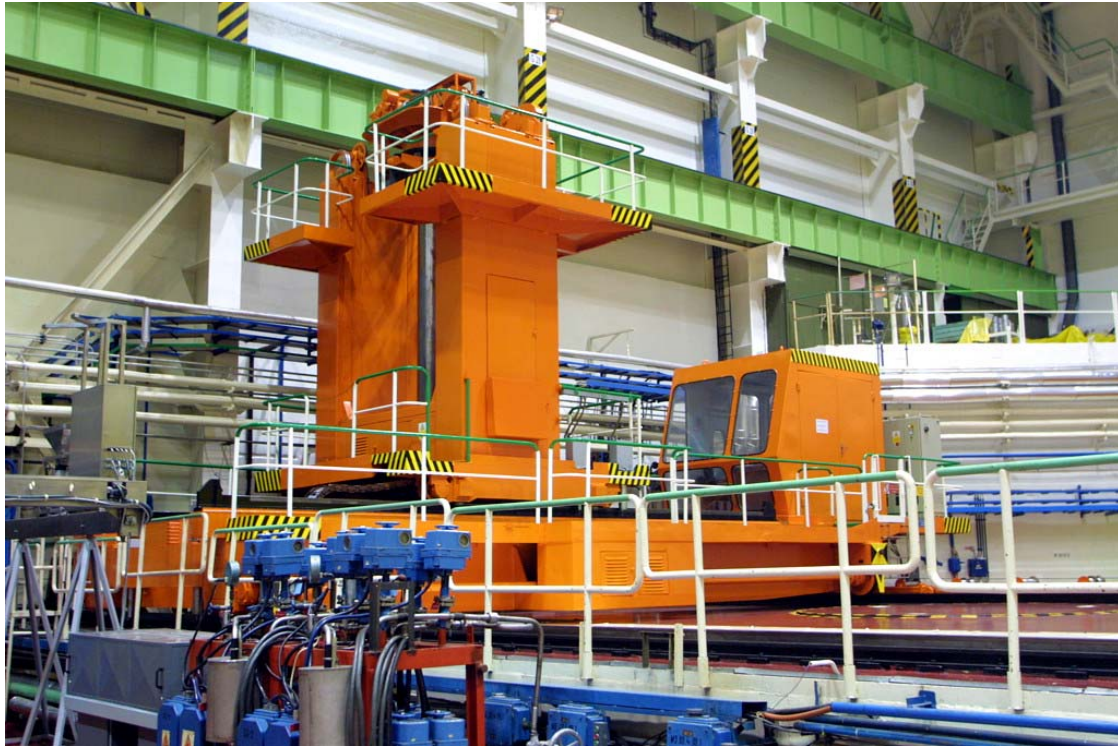
Picture No. 11 V1 Nuclear Power Plant - Refueling machine at fuel replacement
