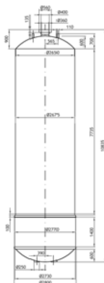
Graph No. 33. Schematic drawing of bubble tank body
