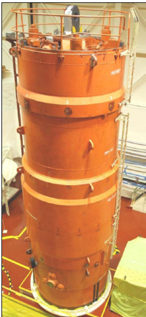
Graph No. 19. General view of the RIS container (KVČR) / Similar Lifting device / Remote Sampling Add attached to the RIS Container KVČR during RIS characterization
