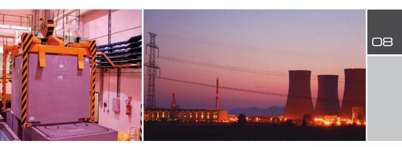
The necessity to build a technology to produce fibre-concrete containers results from the need to process RAW so that is can be safely stored in the National RAW Repository for long period of time avoiding any leakages to the environment. The technology is based on French licence, producing containers from special concrete reinforced with non-corrosive metal fibres appropriate for usage in nuclear industry.
