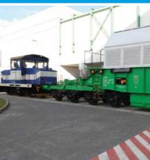
Transport of spent nuclear fuel from VVER 440 type reactors is performed by transport container C-30, including services related to radiation and nuclear safety. The transport set consists of a transport container of the C-30 type, reservoir of the KZ-48 type (T-12 or T-13), and a railway carriage Uaais/Hx of the 9-713.0 type.
