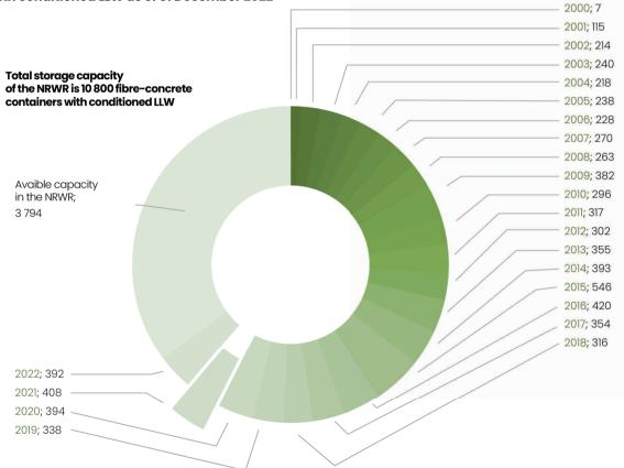
Overview of the filling of the storage capacity of the NRWR by disposing VLLW as of 31 December 2022
